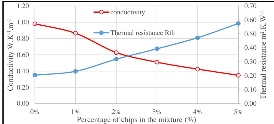
Figure 6: Evolution of conductivity and thermal resistance as a function of the percentage of chips for a 20cm wall
