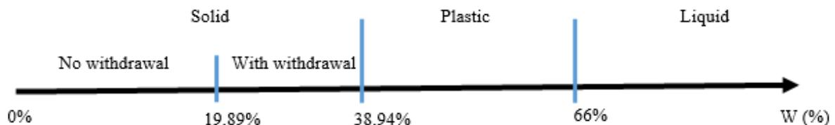
Figure 4: Consistency diagram of clay material
