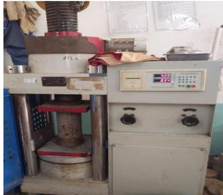
Figure 1: Crushing of a specimen with a hydraulic press
