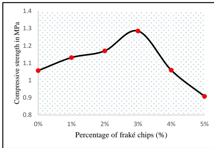
Figure 5: Compressive strength as a function of percentage of chips
