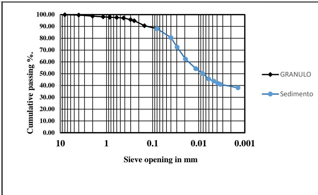
Figure 3: Granulometry + sedimentometry
